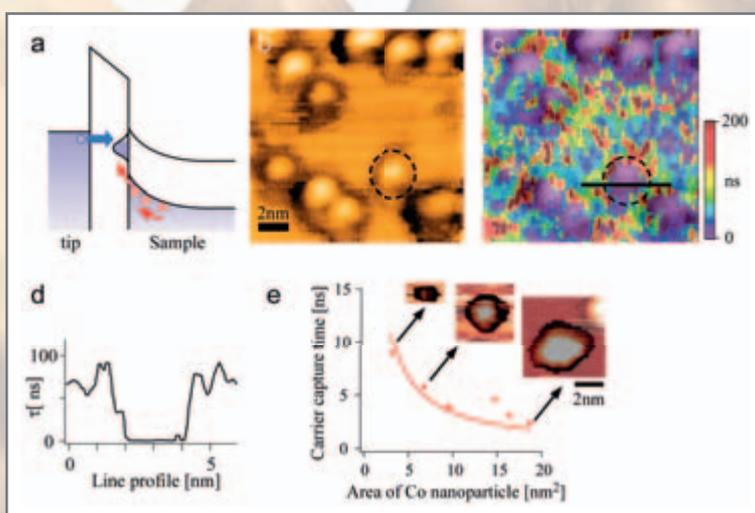
Fig. 3 (a) Schematic of the carrier recombination mechanism via the gap states. (b) STM image of Co nanoparticles/GaAs. (c) Overlap of color-scale two-dimensional mapping of decay constant obtained over the surface in (a). (d) Cross section of the decay constant along the line in (b). (e) Hole capture time as a function of nanoparticle size.
