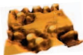
3D representation of the STM image of Co nanoparticles/GaAs
